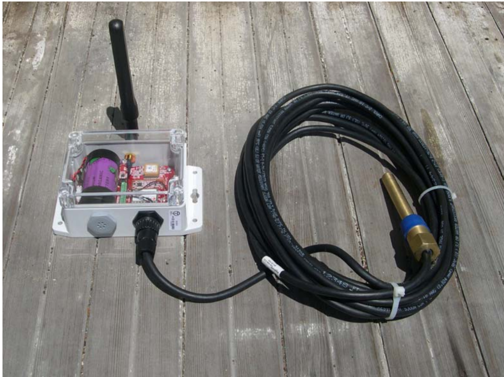
Basic Water Tank Monitor Hardware
